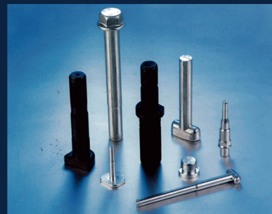
由热激成形改为冷激成形的产品 The product forming is changed from hot upsetting to cold upsetting
